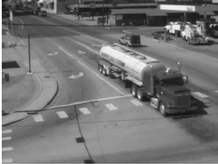
Figure 4. Adjacent-Lane Occlusion with Right-Side Camera.
