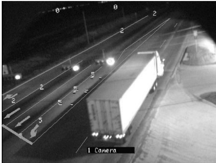
Figure 5. Adjacent-Lane Occlusion with Left-Side Camera.
