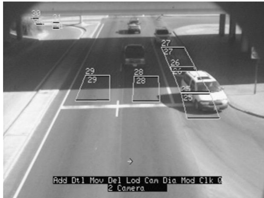
Figure 12. Shadows from Tall Vehicles and Bridge Structures.
